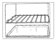
Next, lower the front until the shelf support guides fit onto the support guides located at each side of the oven in the front.
